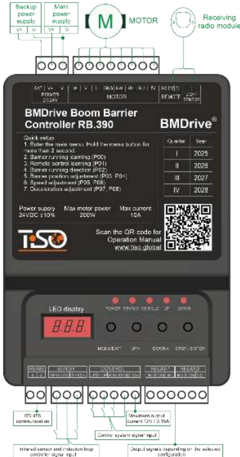
Fig.17 - Terminal designations of the RB390 controller
