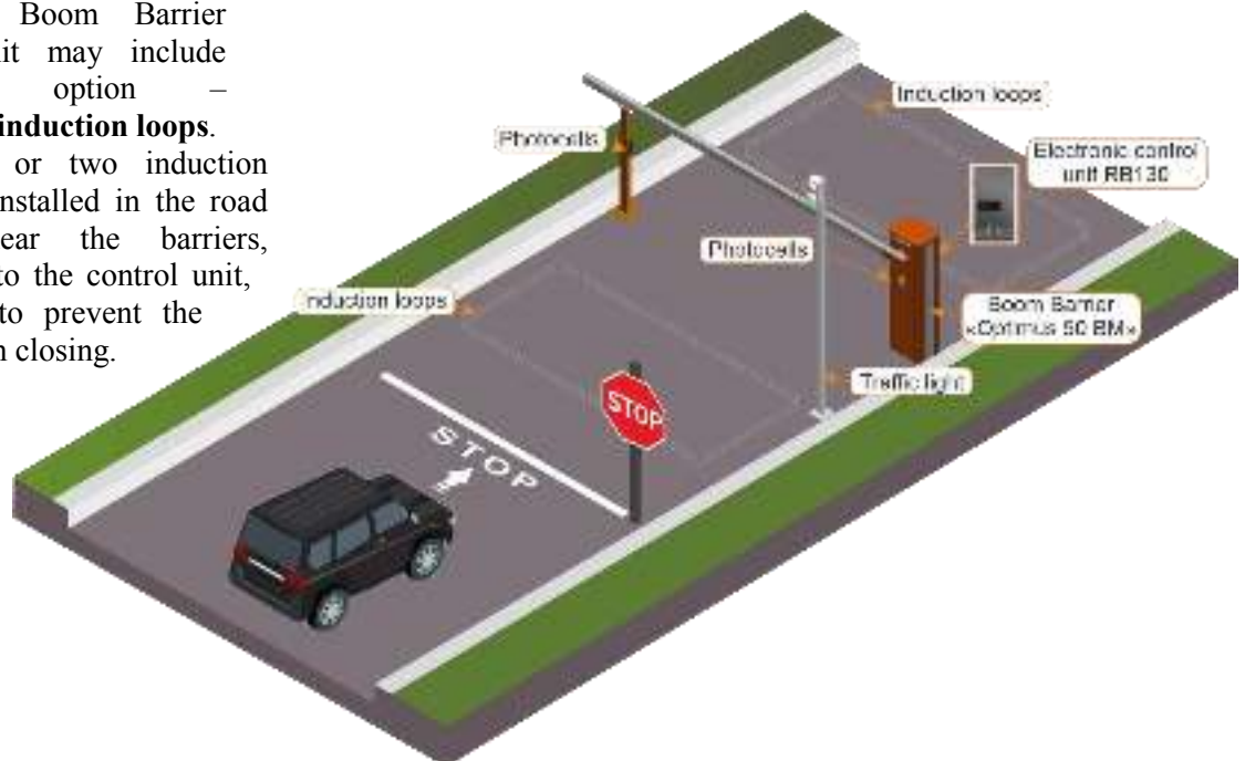
Fig.10 – Induction Loops in design position
